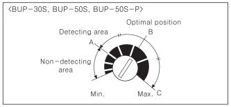
When place a target within detecting range of sensor, turn the VR from minimum position until the LED is turned on or off(Dark on mode/Light on mode), this position is "A". (The LED can be turned on or off where the lowest sensitivity position.)
