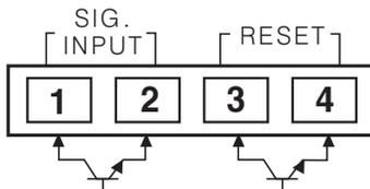
※Please use reliable contacts enough to flow 10 $\mu$ A current when using contact as a input signal or reset signal.
